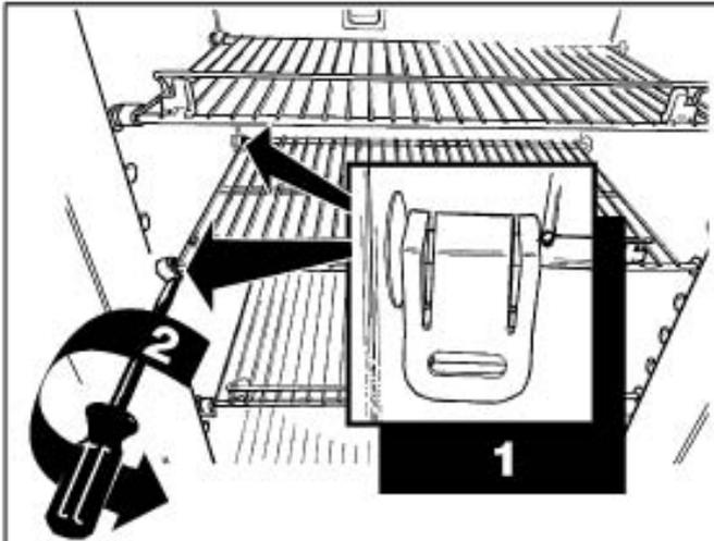
Put a screwdriver into the slot of the shelf lock. Turn the screwdriver counterclockwise. Remove the shelf locks from the wire shelf.
