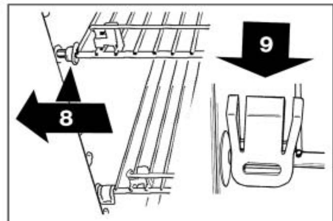
Slide the plastic plugs into the holes of the wall. Snap the shelf locks onto the wire shelf.
