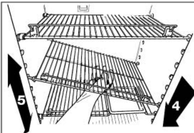
Lower the right-hand side of the wire shelf and let the left-hand side slide out of the holes in the wall.
