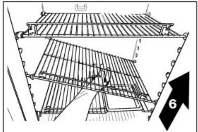
Insert the ends of the wire shelf on the left-hand side at the desired position.
