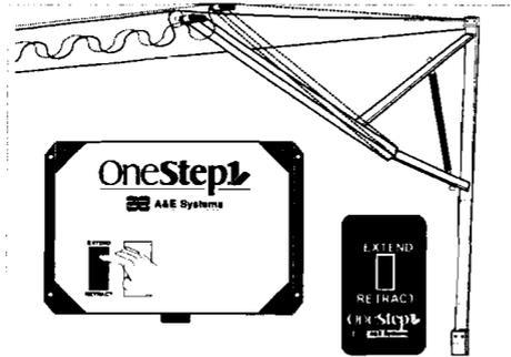
**Note:** The control box system is protected with a 10 amp fuse. If needed, a spare 10 amp fuse is taped inside the control box. Shut off the 12VDC power to control box and remove control box cover to expose fuse on inside. Replace if necessary.
