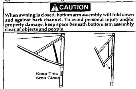
Remove tie downs and sun screen if installed. Press and hold the "RETRACT" button on the control box or the remote switch. When awning is fully closed, release button. **Important: Do not press the control box and the remote switch "Retract" buttons at the same time. Awning will not work and/or may cause control box fuse to blow.**
