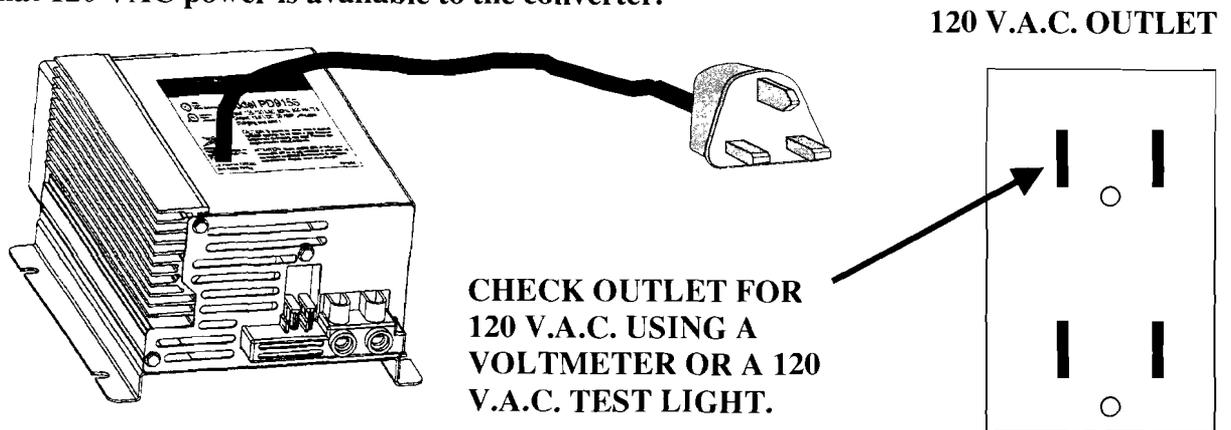
**If the converter fuses are good and 120 V.A.C. power is available at the outlet into which the converter is plugged, and the converter output still reads zero volts, the converter is bad and must be replaced.**
