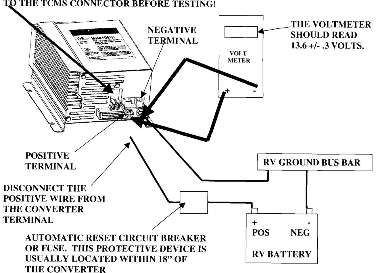
If the converter output voltage reads 13.6 volts, but the battery is still not charging, the problem could be an open automatic reset circuit breaker or open wire between the converter and RV Battery.
