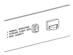
The refrigerator has a storage switch located on the center divider strip between the two doors. This switch <u>must</u> be in the Normal Operation (ON) position or in the High Humidity (ON) position in order for the refrigerator to operate on any mode.
