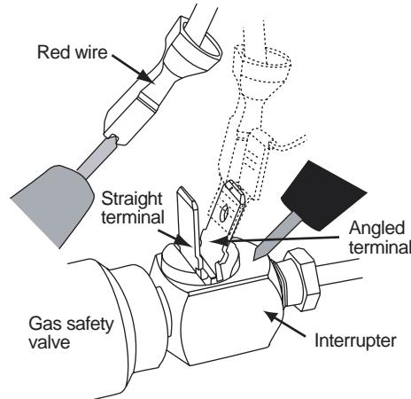
**Figure 6. Checking red wire to ground (see NOTE)**
