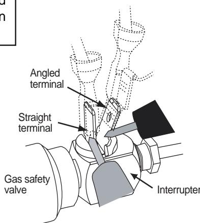
**Figure 7. Checking voltage across terminals (see NOTE)**
