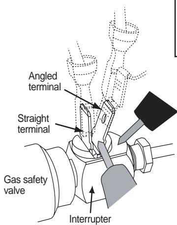
**Figure 5. Checking angled terminal to ground (see NOTE)**
