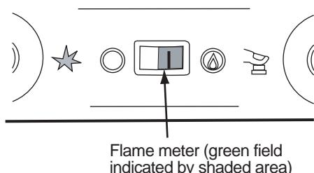
Figure 2. Flame meter indicating a flame is present
