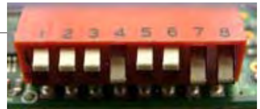
Example Switches set for DISH Network, mount option A.
