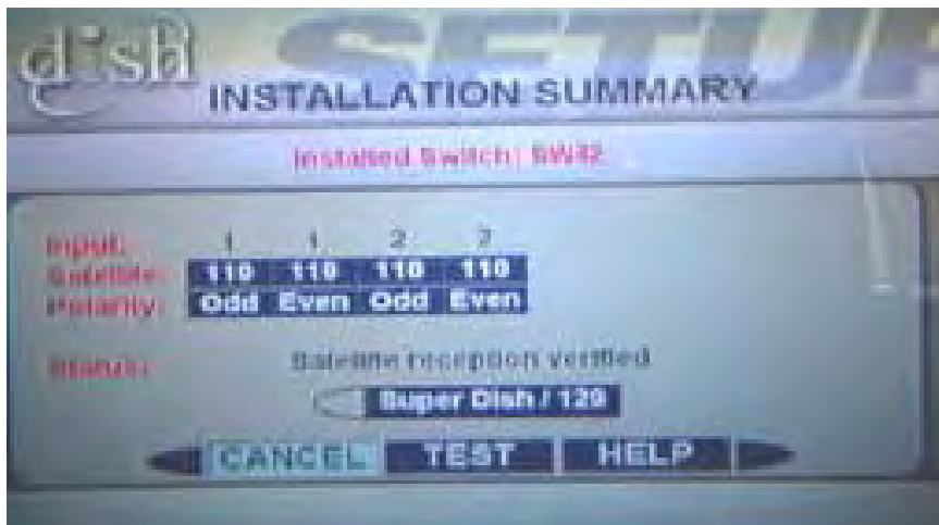
DISH Network Installation Summary Screen
