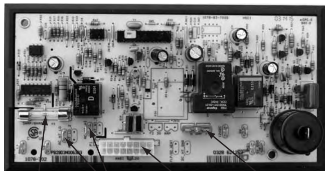
5 amp fuse ac power (F3) AC heater terminals Wire harness connector (P1) 5 amp fuse dc power (F1)
