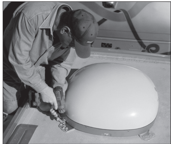
Figure 8 Attaching/Sealing the Mounting Plates
