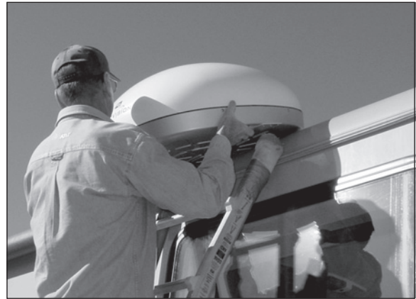
Figure 4 Carrying Antenna to Roof
