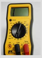
Step 2: Connect multi-meter to float switch wires and actuate the float on the switch.
