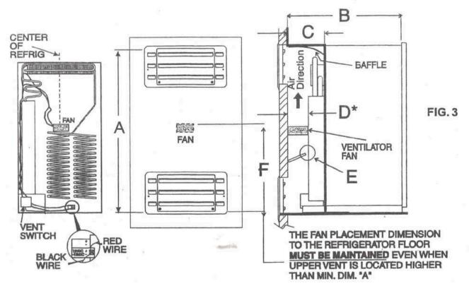
\* When dimension "D" exceeds 1", it may be necessary to add baffle/s above lower access vent, as shown, for more efficient operation in warm temperatures.
