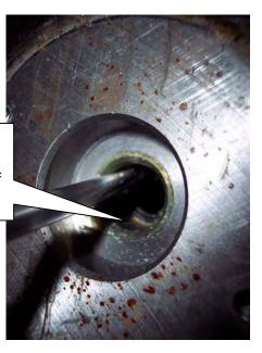
Install the new seal with a socket the same diameter as the seal. Use light taps until the seal is fully seated.
