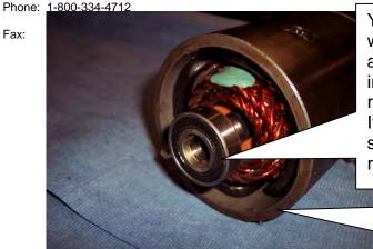
Your motor may come off with or without this bearing still on the armature shaft (it may still be stuck in the port plate). It should be replaced if you replace the motor. If the motor is not badly rusty simply install the new bearing and reassemble.
