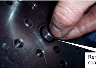
Remove the spacer from the seal area
