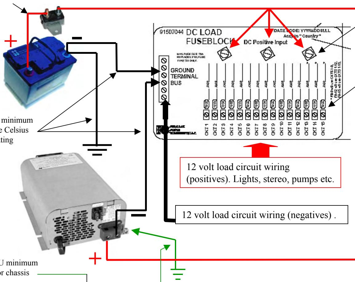
DC Positive Input terminals are electrically connected together and may be used for source DC positive connections as desired.
