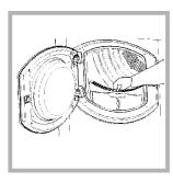
Removing the filter: 1. Pull the plastic grip of the filter upwards (*see diagram*).
