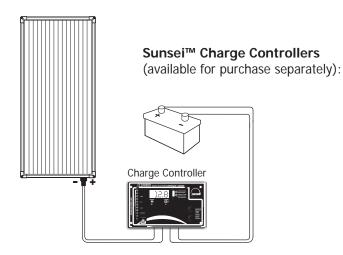
**CC10000:** Two-step charging, overcharge protection; used in systems up to 10A capacity (150W).
