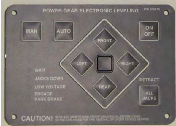
Dewald/Power Gear automatic system touch pad #500629
