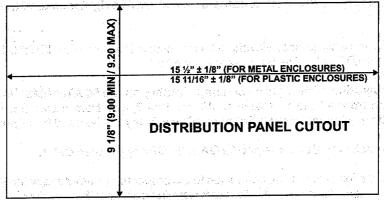
This opening must be cut carefully to be sure the mounting screws will have enough wood to hold and there is enough clearance around the box for the front cover screws.
