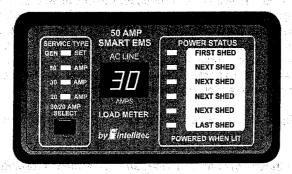
The Display Panel can be mounted remotely and connects to the main unit with a light gauge, three-wire cable. Six Power Status LED's indicate power is applied to those loads. These LED's are on when the power is applied. If 120 VAC service is available, the Load Meter has a two-digit display to *indicate the amount of current actually being drawn* by all the appliances in the coach. If 240 VAC service is available, the two-digit load meter goes blank.
