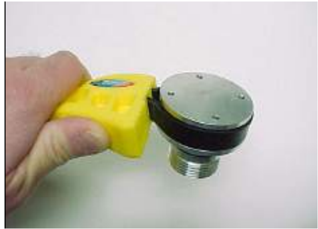
STEP 7A- HR STYLE JACKS WILL USE A PISTON WHICH REQUIRES A STRAP WRENCH TO REMOVE
