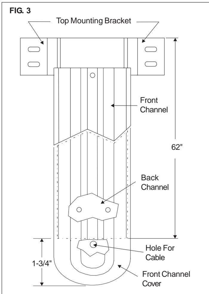
When routing harness, take pre-caution against wires rubbing on sharp edges and use a grommet when going through walls. Harness should be routed so that when the bottom bracket is installed (WeatherPro) it will cover hole where wire goes through wall. Seal any holes with clear silicon sealant. See FIG.3.
