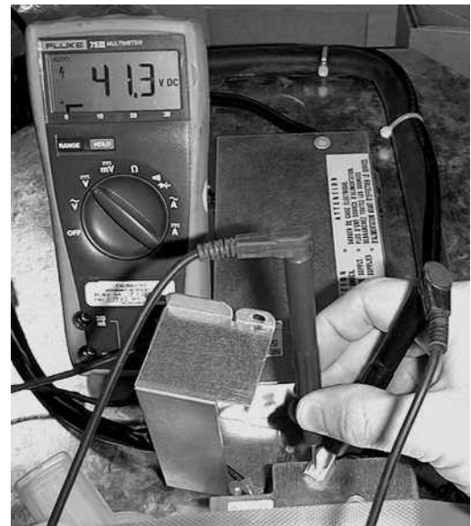
Figure 5 – Measuring AC Power Supply Output
