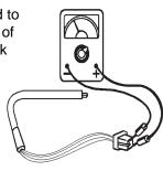
heating element at room temperature. The proper ohms for RM3604 is 48 and RM3804 is 44 with a tolerance of ten percent. If the resistance is outside the tolerance range, replace the heating element.
