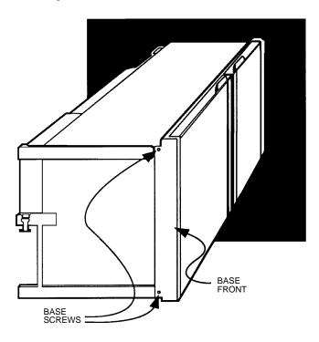
Loosen both screws slightly. Reposition the base until the door is reoriented. Retighten the base screws while holding the base in its new position.
