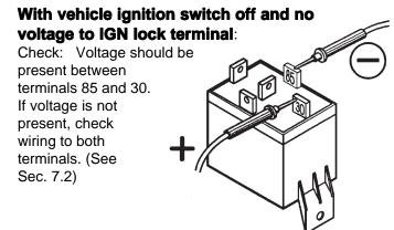
Voltage should **NOT** be present between terminals 85 and 87. If voltage is present, the relay is defective and needs to be replaced.
