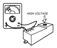
NOTE: If a spark is not produced within 10 seconds, the gas flame warning lamp will illuminate. If spark is produced it will take three minutes for lamp to illuminate. If all of the previous checks are correct, the igniter is good – do not replace.
