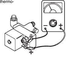
assembly, verify the thermocouple is good (see Sec. 6.3), the tip is clean and the receptacle in the solenoid valve assembly is clean. If the thermocouple checks good, then replace the solenoid valve assembly.
