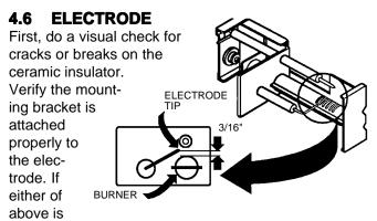
found, replace the electrode. The spark gap must be set at three sixteenths (3/16") of an inch and tip of electrode above the slots in the burner.
