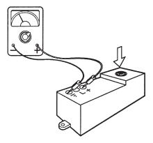
Next, disconnect DC power at refrigerator terminal block. Remove high voltage cable from igniter. Reconnect DC power — the igniter should produce a sparking sound. If not, replace the igniter. With the igniter producing spark, connect meter leads to "L" and ground (–) terminals on the igniter, with the meter set on 20 volts DC range or lower. The meter should read a pulsating voltage. If not, replace the igniter.
