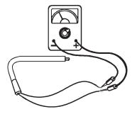
temperature. The proper ohms for RM3604 and RM3804 DC heating element is .67 with a tolerance range of ten percent. If the heating element is outside this range, replace it.
