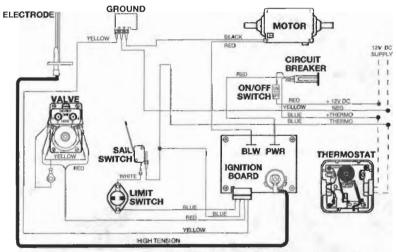
NOTE: DC Models only ON/OFF Switch may be separate or combined in Circuit Breaker.
