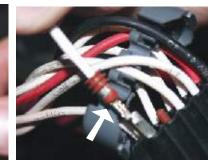
Insert white pin wire from Pressure Sensor Wiring Harness. Snap in to seat.
