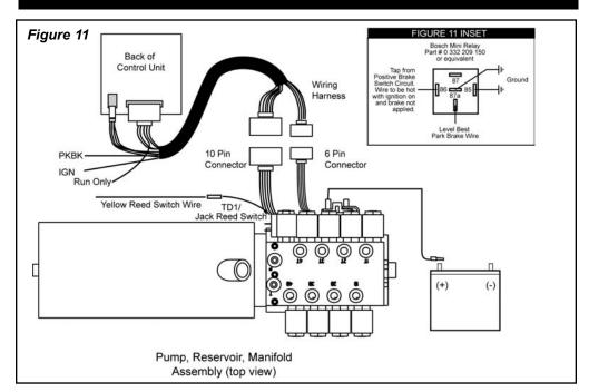
With the wiring from the Control Panel routed to the pump manifold, complete the wire connections. Refer to **Figure 11** for wire connection information.
