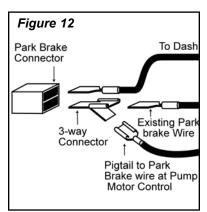
**4.** Level Best systems are equipped with a park brake interlock. The interlock is designed to allow operation of the system only when the vehicle parking brake is set.
