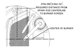
Figure 6 Electrode Adjustment
