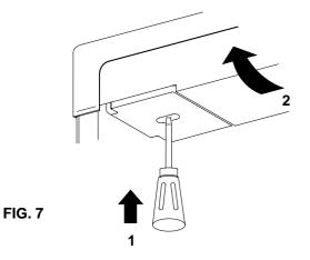
Install the two screws in the top frame, the holes are accessible from underneath.
