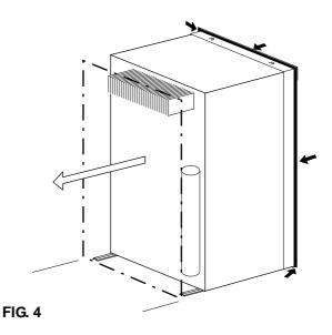
The sealing should provide a complete isolation of the appliance's combustion system from the vehicle interior.
